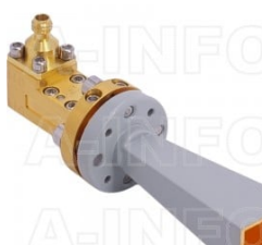
LB-15-15-C-1.0F Standard Gain Horn Antenna 50-75GHz 15dB Gain 1.0mm Female
